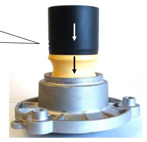
Install the factory top mount and secure it with the supplied nut. Tightening torque for the piston rod nut is 35 Nm (26 ft-lb). The strut unit has to be installed according to manufacturers instructions settings regarding tightening torque and fixing specifications.
