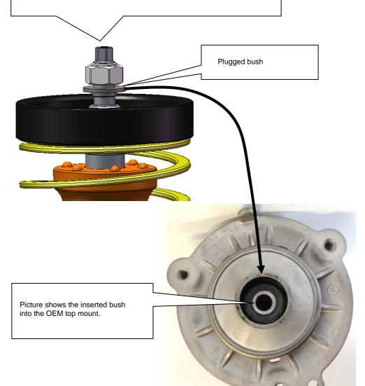
Install the factory top mount and secure it with the supplied nut. Tightening torque for the piston rod nut is 35 Nm (26 ft-lb). The strut unit has to be installed according to manufacturers instructions settings regarding tightening torque and fixing specifications.
