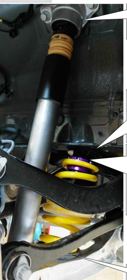
Please install the damper unit to manufacturers recommended settings regarding tightening torque and fixing specifications.
