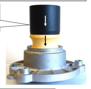
Insert / press in the plugged bush into the top mount.
