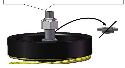
Push the supplied bump stop with dust cover into the original top mount.
