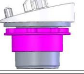
Mount the rear axle adjustment with adapter between spring and chassis, the original spring support is no longer used. You have to remove the rear axle adjustment to correct (screw up the threaded ring) the car height.
