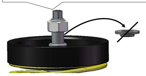
Push the supplied bump stop with dust cover into the original top mount.
