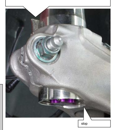
After you have completed installation of the suspension, check the clearance of the tire to the front sus-pension strut. The minimum clearance at the nar-rowest point is 5 mm and must, where necessary, be provided using commercially available, Tech-nical Inspectorate approved spacers.
