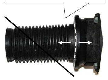
The marks of the OEM upper top mount (upper part) and the OEM axial bearing (bottom part) need to be put on top of each other! The marks show to the vehicle internal side in installed condition.
