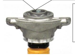
Mount the rear axle adjustment between spring and chassis, the original spring support is no longer used. You have to remove the rear axle adjustment to correct (screw up the threaded ring) the car height. Attention: Before the installation of the height adjustment perch the touching surface area have to be cleaned.
