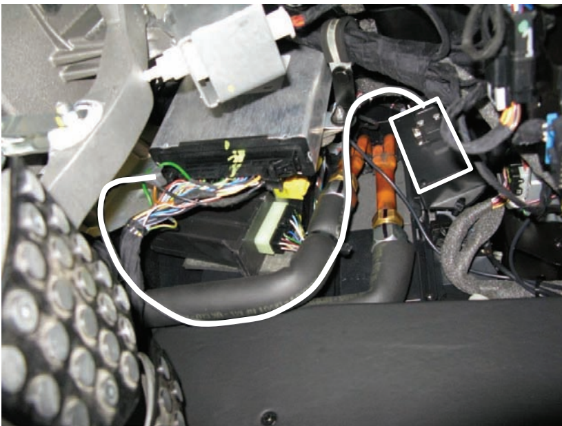
Fix the supplied suspension control unit with cable ties. Connect the suspension control unit on the standard suspension control unit as shown on the connection diagram 1.
