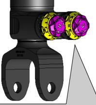
At dampers with compression adjustment, mount the adjustment wheel facing to the rear of the vehicle as shown on the picture.
