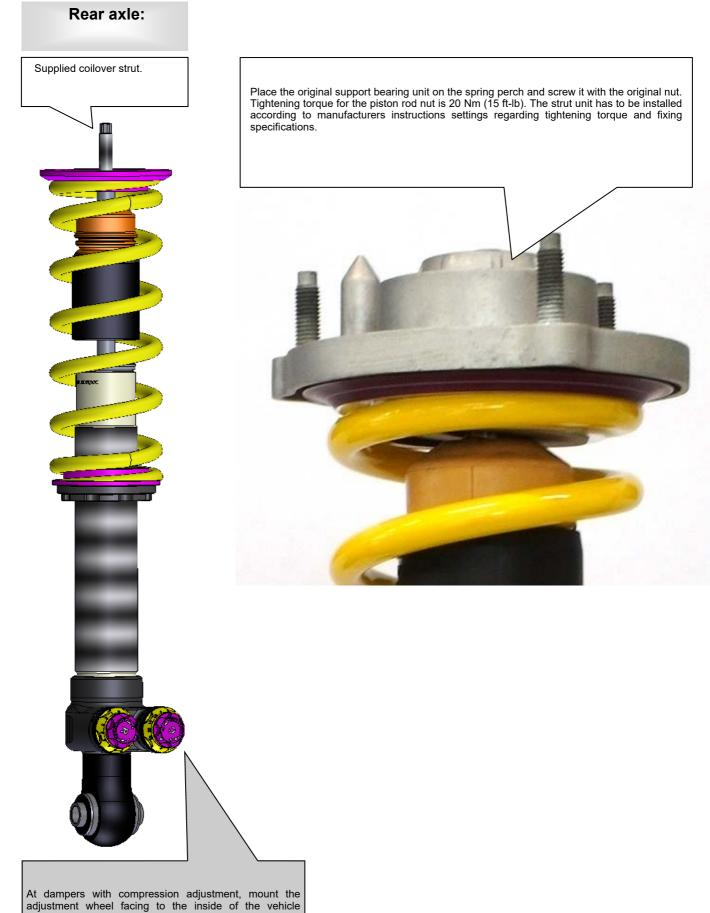
adjustment wheel facing to the inside of the vehicle as shown on the picture.
