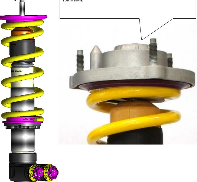
At dampers with compression adjustment, mount the adjustment wheel facing to the rear of the vehicle as shown on the picture.
