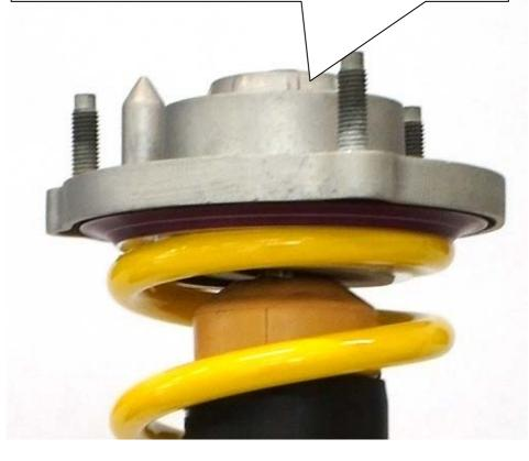
At dampers with compression adjustment, mount the adjustment wheel facing to the inside of the vehicle as shown on the picture.
