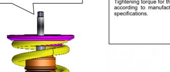
Place the original support bearing unit on the spring perch and screw it with the original nut. Tightening torque for the piston rod nut is 20 Nm (15 ft-lb). The strut unit has to be installed according to manufacturers instructions settings regarding tightening torque and fixing specifications.
