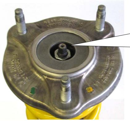
Install the original supporting bearing and fix it with the standard nut. Please install the strut unit to manufacturers recommended settings regarding tightening torque and fixing specifications.
