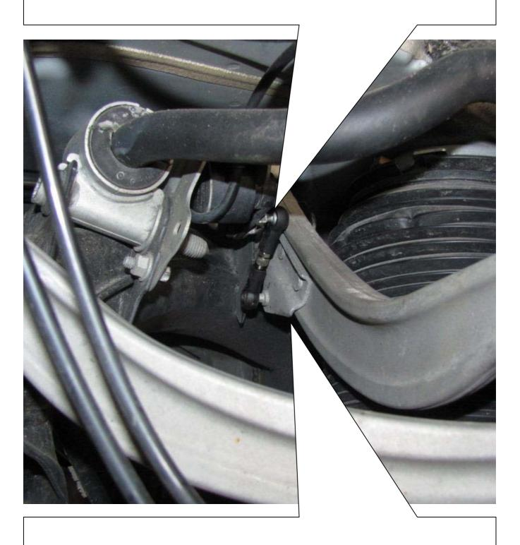
The distance which has to be measured from spherical head centre to spherical head centre should be between 57 mm and 60 mm / 2,24 inch - 2,36 inch. For reaching the distance between wheel centre and fender bending edge on the rear axle you could correct the length of the joint rod. The joint rods must have the same length on both car sides.
