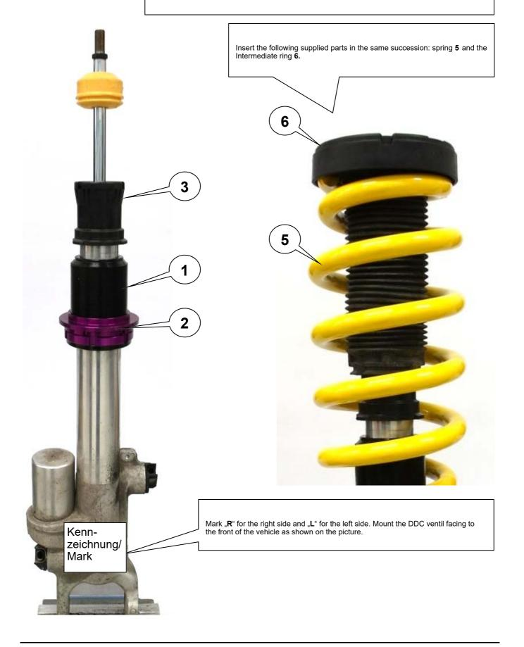
Install the original supporting bearing fix it with the standard nut. Please install the strut unit to manufacturers recommended settings regarding tightening torque and fixing specifications.
