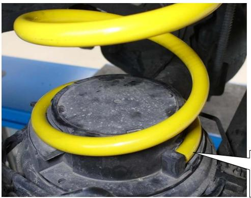
Use the original spring support at the bottom end of the spring.
