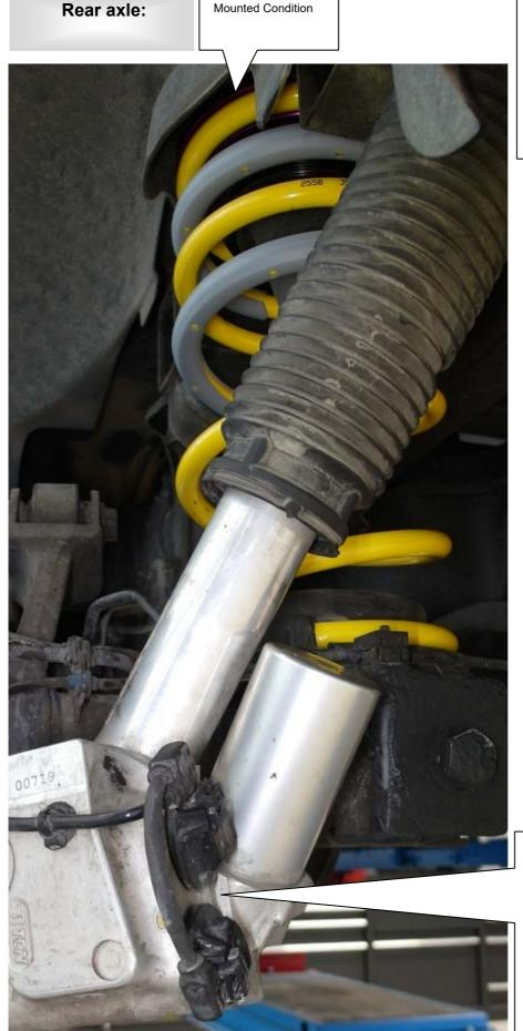
The damper unit and the spring has to be installed according to manufacturers instructions settings regarding tightening torque and fixing specifications.
