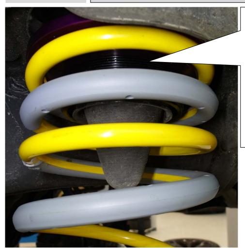
Mount the rear axle adjustment between spring and chassis, the original spring support is no longer used. You have to remove the rear axle adjustment to correct (screw up the threaded ring) the car height.
