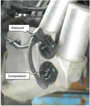
Remove the standard top mount, spring, spring perch, bumpstopp, dust cover and the protection cap. Then thoroughly clean the damper!
