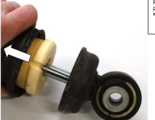
Pull down the dust cover and stop element and mount the supplied piston rod clamp on the damper. Then dismantle the upper damper eye.
