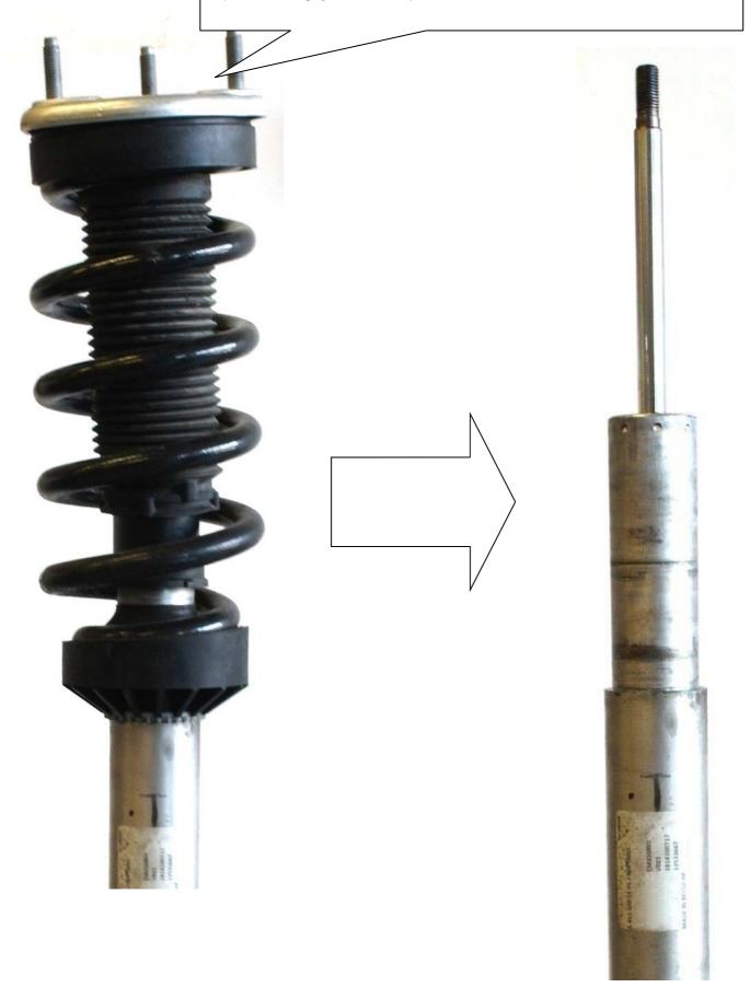
Insert the supplied threaded bush  ${\bf 1}$  with, threaded ring  ${\bf 2}$  the ventilation cap  ${\bf 3}$  and the new bumpstopp  ${\bf 4}$  on the coilover strut.
