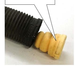
Attach the supplied bump stop element on the damper. The OEM bump stop is no longer required and must be dismantled.
