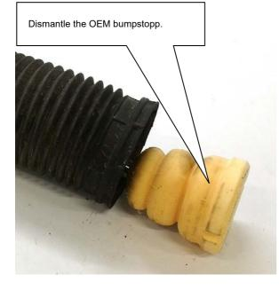
Attach the supplied bump stop element on the damper. The OEM bump stop is no longer required and must be dismantled.
