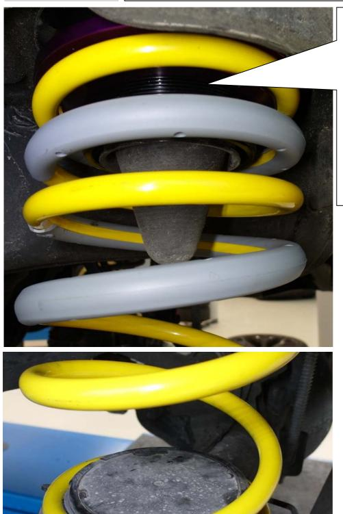
Mount the rear axle adjustment Mount the rear axle adjustment between spring and chassis, the original spring support is no longer used. You have to remove the rear axle adjustment to correct (screw up the threaded ring) the car height. Attention: Before the installation of the height adjustment perch the touching surface area have to be
