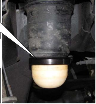
Tightening torque for the bottom damper nut is 40 Nm (29 ft-lb). The damper unit has to be installed according to manufacturers instructions settings regarding tightening torque and fixing specifications.
