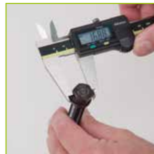
d Measure the hexagon of the spindle head.
