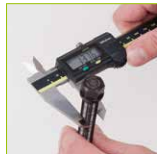
a Measure the spindle diameter.
