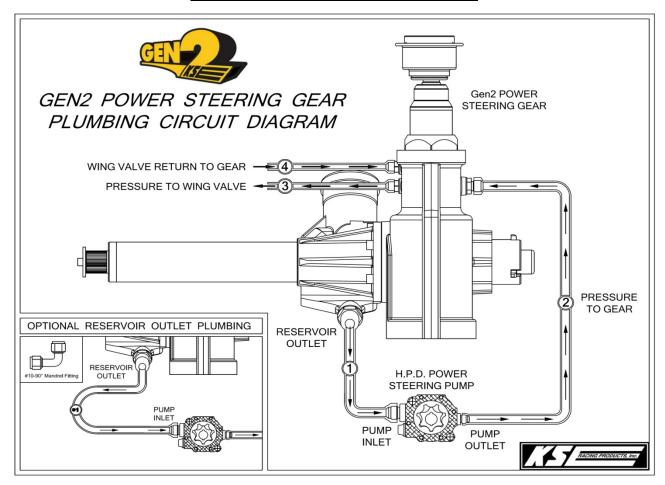
*IMPORTANT:* All hoses and fittings must be clean and free of all contamination. It is highly recommended that these components be flushed with clean solvent or hot soap and water and blown dry before assembly. When installing hoses, take care to assure that they will not be exposed to being pinched, cut or rubbed that would cause hose damage or failure, which could cause poor power steering performance or failure.
