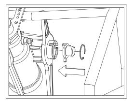
**STEP 8** Tighten output tube mounting bracket. It is not recommended to float this mounting point with the inboard mounting system.
