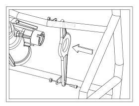
**STEP 5** Slide Gen2 steering gear into inboard mounting bracket.
