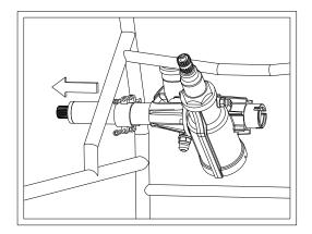
**STEP 4** Install inboard mounting bracket P/N KSC1070 or equivalent, on chassis mounting tabs. Depending on tab locations, either side is acceptable.
