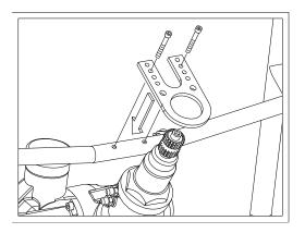
**STEP 7** Install inboard mount retaining cap and snap ring.
