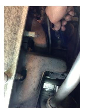
3. Next generously soak the bolts holding the downpipe to the cat back exhaust section (this particular car already had an aftermarket exhaust which was replaced with a Krona Performance Turbo back ©)
