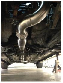
9. Make sure all connections are completely seated and tighten clamps at the actual connection points (on the areas where the pipe is relief cut. There should be no overlap of pipe. \*torque clamps to 20 ft-lb's
