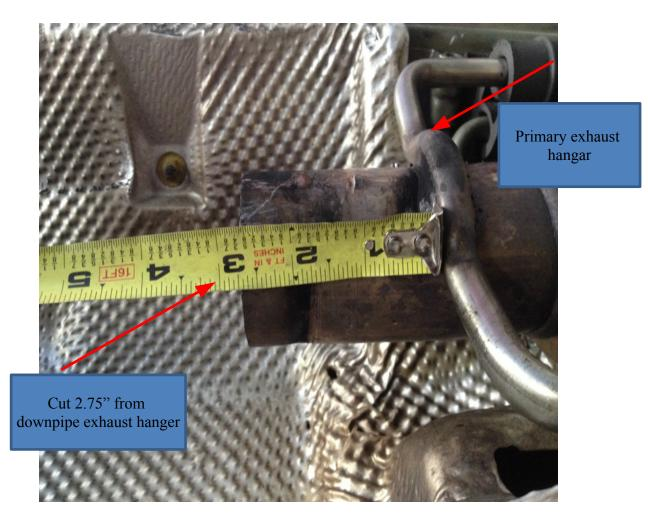
There are only 6 rubber exhaust hangers holding the OE exhaust to the vehicle (two at the OE downpipe after the flex joint, one just after the center resonator, one just before the rear muffler and two on the rear muffler. Remove the exhaust from the downpipe back by slipping the factory hangars from the rubber mounting points. With a little bit of elbow grease you can slide the factory system out from under the vehicle (If all else fails talk nice to it;-))
