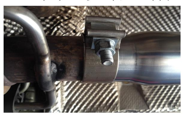
5. Next you may move to connecting the 3" resonator section to the Krona adapter pipe. Be sure to slip a 3" clamp over the end of the adapter pipe before making the connection.
