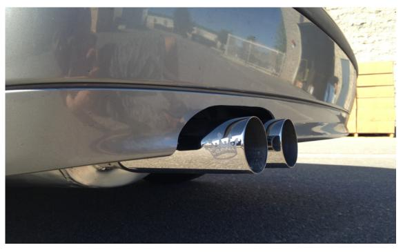
Position the muffler so that it is center perfectly in the bumper cut out. Once you are happy with its location you may now tighten all exhaust clamps starting with the muffler and working your way forward. **Torque all slip fit connections to 20 ft lbs.**
