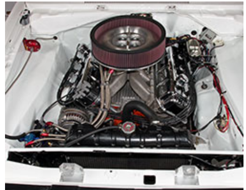
K&N 14" spun aluminum air cleaner kit, 85-6851, will work with 2-5/16", 3", 4", 5", and 6" tall K&N air filters as well as several other variations for drag racing & off-road racing use
