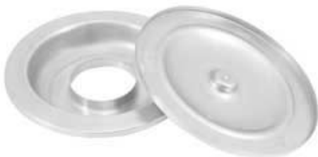
K&N's lightweight spun aluminum air cleaners feature a drop base plate which drops the base of the air filter 1-1/2 inches below the carb flange to maximize hood clearance
