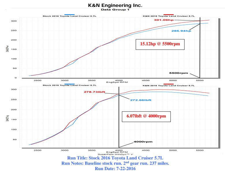
Run Title: K&N 2016 Toyota Land Cruiser 5.7L Run Notes: K&N intake kit #77-9040 installed. 2<sup>nd</sup> gear run. Run Date: 7-22-2016
