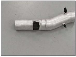
27. Install the mass air sensor into the K&N® intake tube and secure with the provided hardware.
