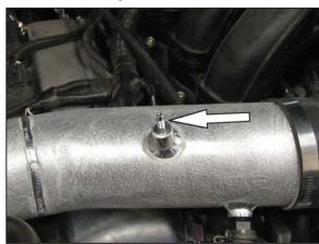
33. Install the engine cover mounting stud into the  $K\&N^{\scriptsize @}$  intake tube.
