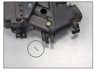
32. Remove the engine cover mounting stud from the air filter housing.
