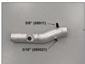
25. Install the provided vent fittings into the K&N® intake tube as shown.
