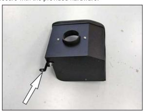
15. Install the heat shield mounting bracket (07958) onto the heat shield as shown using the provided hardware
