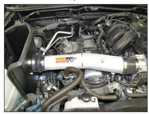
28. Install the K&N® intake tube into the silicone hose at the filter adapter far enough to gain clearance into the silicone hose at the throttle body, then install the tube into the throttle body silicone hose and secure it with the provided hose clamps. NOTE: Do not completely tighten at this time.
