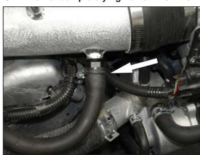
29. Connect the crank case vent hose to the fitting installed into the K&N® intake tube.
