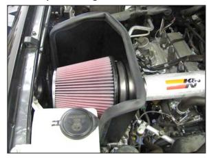
35. Install the K&N $^{\!\scriptscriptstyle \odot}$  air filter and secure with the provided hose clamp.
