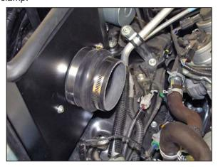
24. Install the provided silicone hose (084079) onto the filter adapter and secure with the provided hose clamp.
