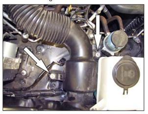
6. Remove the two bolts securing the intake resonator to the inner fender and then remove the intake tube/resonator assembly from the engine compartment.
