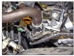
3. Release the spring clamp securing the secondary air hose and then disconnect the secondary air hose.
