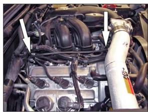
30. Connect the provided fuel pressure vent hose to the fuel pressure regulator and then connect the open end to the fitting installed into the K&N® intake tube.
