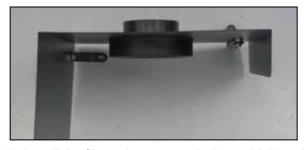
12. Install the filter adapter onto the heat shield and secure with the provided hardware.
