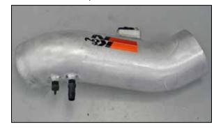
19. Install the provided NPT vent fittings into the  $K\&N^{\circ}$  intake tube as shown.
