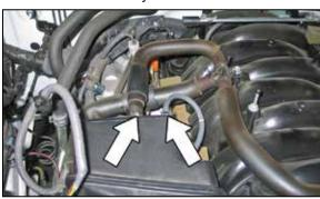
5. Disconnect the crank case vent hose and fuel pressure line from the intake resonator.
