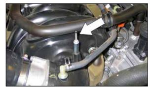
29. Install the mounting stud into the nut extension as shown.
