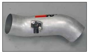
18. Install the mass air sensor into the intake tube and secure with the provided hardware.
