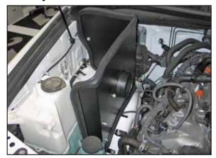
14. Set the heat shield into the engine compartment and secure the factory install nuts with the provided hardware.
