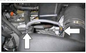
2. Disconnect the mass air sensor electrical connection and then unhook the wiring harness from the air box.
