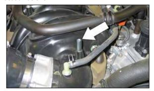
28. Install the provided nut extension onto the stud as shown.
