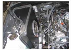
19. Set the heat shield into position on the inner fender and then secure with the factory bolt removed in step #18 and the provided hardware. **NOTE: Be sure to place the ground strap between the inner fender and bracket.**
