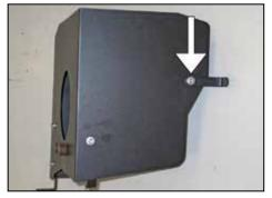
14. Install the provided heat shield mounting
