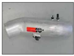
22. Install the provided NPT fittings into the K&N $^{\mbox{\scriptsize \$}}$  intake tube as shown.
