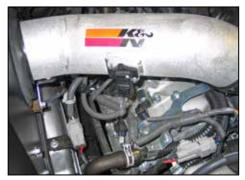
30. Reconnect the mass air sensor electrical connection.
