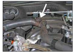
4. Disconnect the crankcase vent hose from the TEE fitting on top of the intake manifold plenum.
