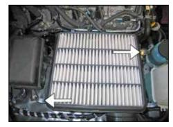
9. Loosen the two bolts securing the lower airbox into the vehicle.
