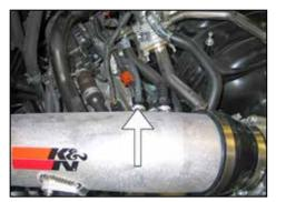
28. Reconnect the fuel pressure regulator vent line to the NPT fitting as shown.
