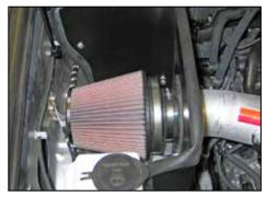
27. Install the filter assembly onto the K&N<sup>®</sup> intake tube and secure with the provided hose clamp.
