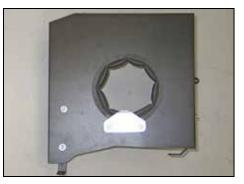
16. Install the provided shorter edge trim into the hole of the heat shield as shown.
