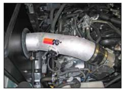
24. Install the K&N<sup>®</sup> intake tube into the silicone hose at the throttle body and align with the mounting bracket attached to the heat shield. Secure the intake tube with the provided hardware and hose clamp.
