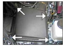
7. Release the four latches' securing the upper airbox to the lower airbox.
