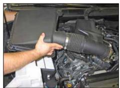
2. Lift up the engine cover to dislodge it from the mounting studs and then remove the engine cover from the vehicle.
