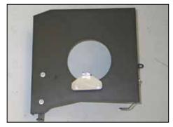
15. Install the tube mounting bracket (083152) onto the rubber mounted studs as shown using the provided hardware.
