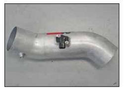
21. Install the mass air sensor into the K&N<sup>®</sup> intake tube and secure with the provided hardware.
