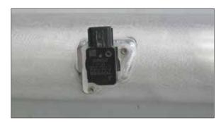
23. Install the mass air sensor into the K&N $^{\circ}$  intake tube and secure with the provided hardware.
