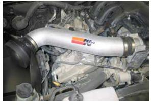
26. <u>Install the intake tube into hump hose</u> at the filter adapter and then into the silicone hose at the throttle body, align the tube for proper fit and then tighten the hose clamps.
