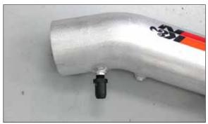
24. Install the 5/8 vent fitting into the K&N $^{\! \rm 8}$  intake tube as shown.
