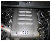
29. Reinstall the engine cover onto the engine.
