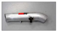
20. Install the mass air sensor into the K&N® intake tube using the hardware provided.
