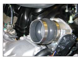
21. Install the silicone hose (084057) onto the throttle body as shown and secure with the provided hose clamp.
