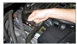
4. Disconnect the crank case vent hose from stock intake tube as shown.
