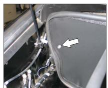
18. Secure the rear heat shield bracket installed during step #14 to the heat shield with the provided spacer and hardware.
