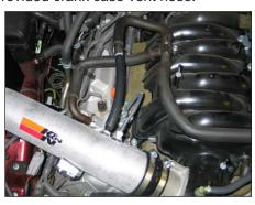
25. Connect the hose mender from the crank case vent hose assembly into the factory crank case vent hose and secure with the factory spring clamp. Then connect the open end to the K&N® intake tube as shown.
