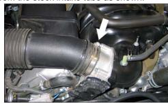
6. Loosen the hose clamp which secures the stock intake tube to the throttle body.
