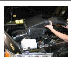
8. Remove the complete stock intake assembly from the vehicle as shown.
