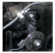
14. Install the small "L" bracket (070742) onto the inner fender using the hardware provided as shown. NOTE: On vehicles equipped with the security system horn, be sure to install the "L" bracket over the horn bracket.
