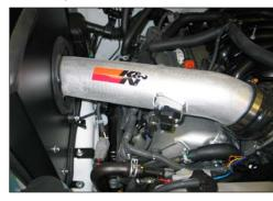
22. Install the K&N® intake tube into the silicone hose at the throttle body and align with bracket installed on the heat shield. Align tube and heat shield then tighten the heat shield and secure the intake tube with the provided hardware.
