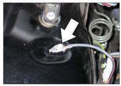
15. Remove the bolt which secures the ground strap to the inner fender.
