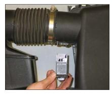
19. Remove the two bolts which secure the mass air sensor into the stock air filter housing and then remove the mass air sensor as shown.
