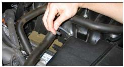
5. Disconnect the fuel pressure regulator vent hose from the stock intake tube as shown.
