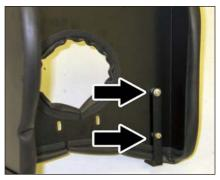
11. Install the large "L" (070902) bracket onto the heat shield as shown using the provided spacers and hardware.
