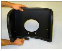
9. Install the large edge trim onto the heat shield as shown.
