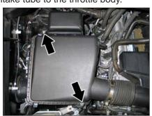
7. Loosen the two bolts which secure the air box to the inner fender.
