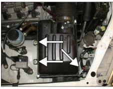
6. Loosen the three bolts that secure the stock air box assembly to the inner fender.
