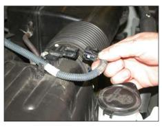
2. Disconnect the mass air sensor electrical connec-
