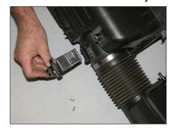
9. Remove the two screws which secure the mass air sensor to the factory air box, then remove the mass air sensor form the air box as shown.
