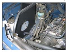
17a. Install the tube mounting bracket (083113) onto the heat shield as shown using the provided hardware.
