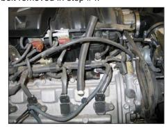
21. Remove the factory crankcase vent hose and fuel pressure regulator vent hose shown from the engine.
