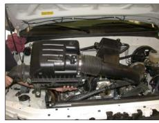
8. Remove the complete intake assembly from the vehicle as shown.
