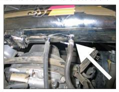
24. Attach the power steering pressure switch vent hose to the K&N® intake tube as shown.
