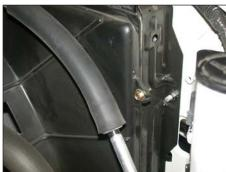
15. Remove the radiator fan shroud upper mounting bolt shown.
