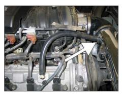
22. Install the provided crankcase vent hose onto the valve cover and then attach to the intake tube as shown.
