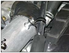
20. Attach the A/C hose to the intake tube with the bolt removed in step #4.
