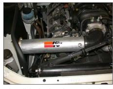
19. Install the intake tube onto the throttle body and align the tube mounting bracket with the threaded boss on the engine, then secure with the provided hardware.
