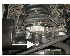
4. Loosen and remove the bolt that secures the A/C hose to the stock intake tube.
