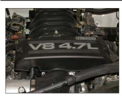
28. Reinstall the engine cover and secure it with the factory mounting nuts removed in step #3.
