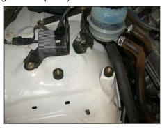
14. Install the two rubber mounted studs to the original air box mounting holes as shown.
