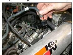
29. Reconnect the mass air sensor electrical connection as shown.
