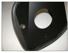
12. Install the rubber mounted stud onto the heat shield as shown using the provided hardware.
