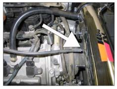
23. Install the provided fuel pressure regulator vent hose onto the fuel pressure regulator and then attach to the K&N® intake tube as shown.
