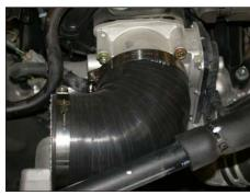
18. Install the silicone hose (084088) onto the throttle body and secure with the provided hose clamp as shown.
