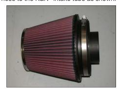
25. Install the filter adapter into the air filter as shown and secure with the provided hose clamp. NOTE: Drycharger® air filter wrap; part number RF-1042DK is available to purchase separately.
