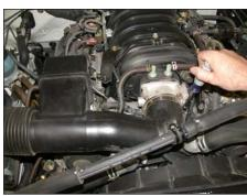
5. Loosen the hose clamp, which secures the stock intake tube to the throttle body.
