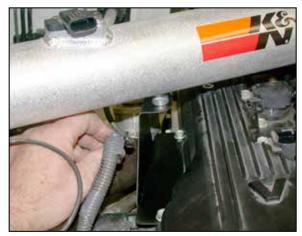
26. Clip the mass air sensor wire harness retainer into the tube-mounting bracket as shown.
