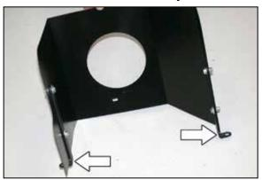
8. Install the two heat shield brackets (07159) onto the heat shield as shown with the provided hardware.
