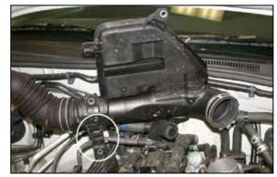
6. Disconnect the wire harness-retaining clip shown from the intake plenum.
