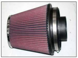
23. Install the radius filter adapter into the K&N<sup>®</sup> air filter and secure with the provided hardware as shown.
