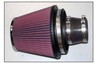
24. Install the provided silicone hose (084055) onto the K&N® air filter and secure with the provided hose clamp as shown.
