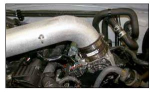
18. Install the K&N<sup>®</sup> intake tube onto the throttle body and align with the tube mounting bracket that was installed in step #14.
