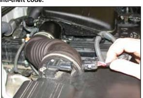
2. Disconnect the mass air sensor electrical connection and unclip the three wire harness retaining clips from the intake plenum.
