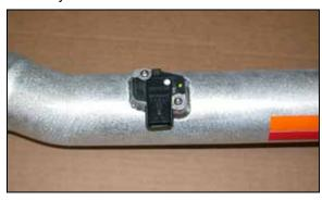
17. Install the mass air sensor into the K&N® intake tube and secure with the provided M4 button head allen bolts as shown.
