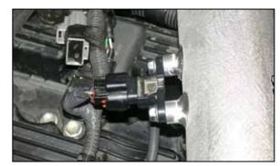
22. Install the pressure sensor onto the K&N® intake tube using the bolts removed in step #3.
