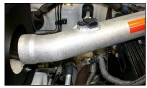
19. Secure the K&N® intake tube to the tube mounting bracket with the provided hardware and then tighten the hose clamp at the throttle body.
