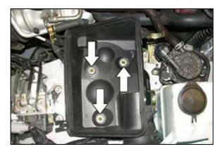
7. Remove the three lower air box retaining bolts shown and then remove the lower air box from the vehicle
