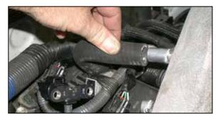
21. Install the provided crank case vent hose onto the valve cover port and then onto the K&N<sup>®</sup> intake tube as shown.
