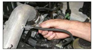
20. Install the provided vacuum hose onto the fuel pressure regulator and then onto the  $K\&N^{\otimes}$  intake tube as shown.
