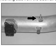
21. Install the engine cover-mounting stud into the K&N® intake tube as shown.
