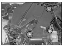
10. Loosen the hose clamp at the throttle body, then remove the two bolts that secure the air box to the engine.
