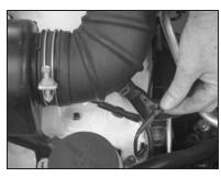
4. Pull the wire harness clip up to release it from the intake tube.
