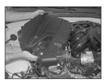
11. Remove the air box assembly from the engine as shown.
