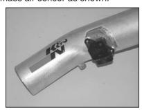
19. Install the mass air sensor into the  $K\&N^{\otimes}$  intake tube as shown using the provided hardware.
