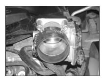
17. Install the silicone hose (08434) onto the throttle body with the provided hose clamps as shown
