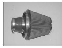
27. Install the provided silicone hose (084055) onto the air filter assembly and secure with the provided hose clamp as shown.
