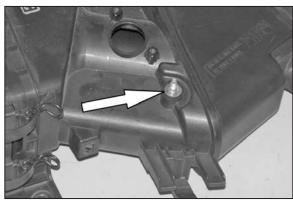
23. Remove the engine cover mounting stud shown from the factory airbox.
