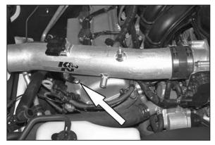
26. Install the K&N<sup>®</sup> intake tube onto the throttle body, align the mounting bracket with the threaded boss on the engine valve cover and then secure with the provided hardware and hose clamp.
