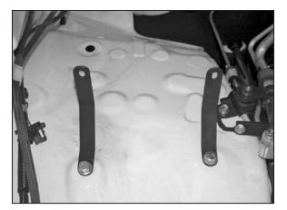
15. Mount the two provided brackets onto the vehicle with the provided hardware. NOTE: Bracket (07172) mounts closest to engine.
