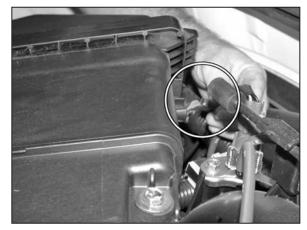
9. Remove the fuel pressure regulator hose from the back side of airbox.
