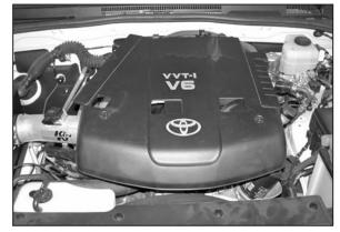
32. Reinstall the engine cover using the original nuts removed in step #1.
