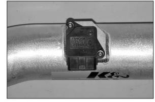
22. Secure the mass air sensor to the  $K\&N^{\circledast}$  intake tube using the provided bolts as shown.
