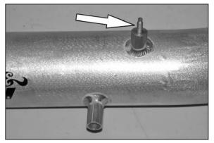
24. Install the stud removed in step #23 into the threaded boss on the  $K\&N^{\mbox{\tiny B}}$  intake tube as shown.
