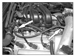
27. Remove the stock vacuum hose from fuel pressure regulator. Install the provided silicone hose, attaching the hose to the fuel pressure regulator and the K&N<sup>®</sup> intake tube nipple.
