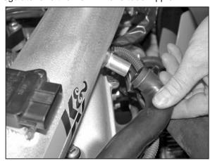
28. Connect the factory crankcase vent hose onto the K&N<sup>®</sup> intake tube as shown.
