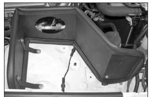
17. Install the heat shield onto the vehicle, then secure the brackets with the provided hardware.
