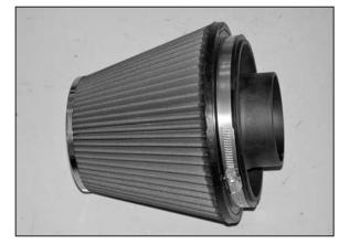
29. Install the filter adapter into the air filter as shown, secure with the provided hose clamp.
