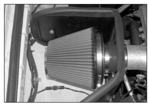
31. Install the air filter assembly onto the K&N<sup>®</sup> intake tube and secure with the provided hose clamp.
