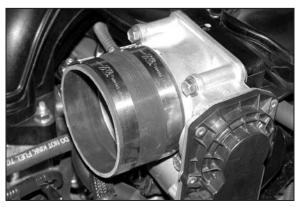
20. Install the provided silicone hose (08434) onto the throttle body with the provided hose clamps.
