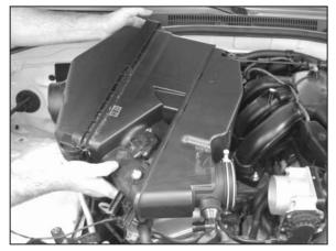
11. Remove the airbox assembly from engine as shown.
