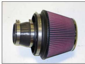
25. Install the silicone hose (084091) onto the filter adapter and secure with the provided hose clamp as shown.
