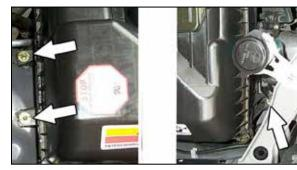
6. Loosen the three bolts that secure the air box assembly.
