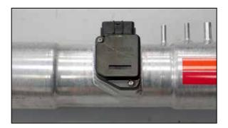
10. Install the mass-air sensor into the K&N $^{\odot}$  intake tube, and secure with the provided screws as shown.
