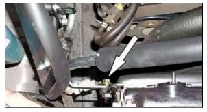
16. Secure the upper bracket to the fan shroud with the original bolt.
