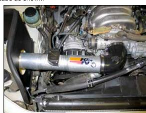
20. Install the K&N® intake tube into the silicone hose at the throttle body and then align the tube mounting bracket with the threaded boss on the engine valve cover. Secure the tube with the provided hardware and tighten the hose clamp.
