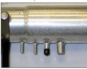
19. On vehicles that are not equipped with the 4th vacuum line, install the provided plug onto the vent tube as shown.
