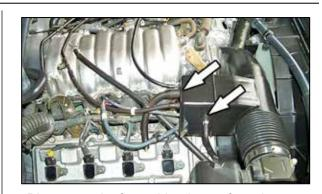
7. Disconnect the four rubber hoses from the engine as shown by the arrows.
