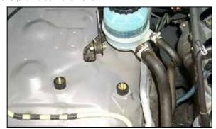
14. Install the two remaining rubber mounted studs to the original air box mounting holes.
