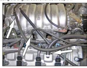
22. Replace the crank case vent line, EVAP vent line, and fuel pressure vent line with vent lines supplied.
