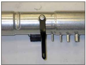
18. Install the tube mounting bracket onto the K&N® intake tube with the provided hardware as shown.
