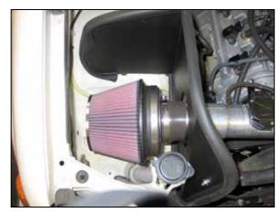
26. Install the air filter assembly onto the  $K\&N^{\otimes}$  intake tube as shown.
