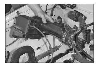
7. Loosen the hose clamp at the throttle body and remove the remaining section of the intake assembly.
