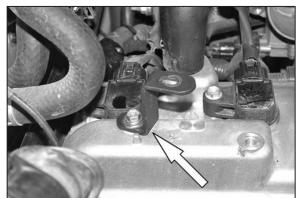
9. Install the "Z" bracket onto the engine using the throttle cable bracket mounting bolt removed in step #8 as shown.
