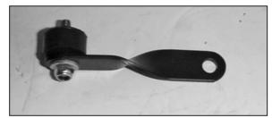
14. Assemble the rubber bumper stud onto the twist bracket with the provided hardware as shown. **NOTE: Do not tighten completely**.
