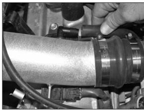
22. Vehicles equipped with the idle air vent line, reconnect vent line as shown.
