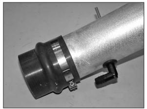
21. Install the 90 degree fitting into the intake tube as shown.
