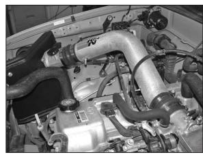
18. Install the intake tube onto the throttle body, then install onto the mass air sensor.
