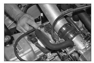
23. Install the provided silicone hose onto the fuel pressure regulator and connect the other end to the  $K\&N^{@}$  intake tube as shown.
