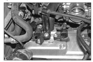
10. Install the throttle cable bracket onto the "Z" bracket installed in step #9 with the provided hardware and reattach the throttle cable to the mounting bracket as shown.
