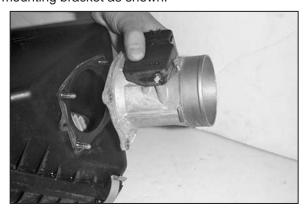
11. Loosen and remove the four hex nuts that secure the mass air sensor to the air cleaner assembly then remove the mass air sensor as shown.
