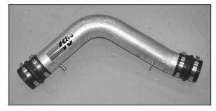
17. Secure the hump hose #08696 to the mass air sensor end of the tube and hump hose #08421 to the throttle body end of the tube as shown with the hose clamps provided.
