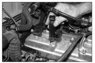
8. Unhook the throttle cable from the hold down bracket and remove the bracket mounting bolt and bracket from the engine as shown.
