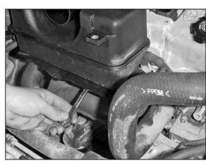
5. Loosen and remove the two nuts that secure the resonator.
