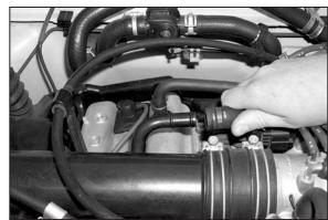
6. Vehicles equipped with an idle air vent line, disconnect vent line as shown.
