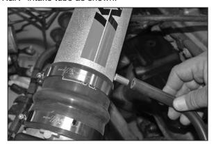
24. Install the provided silicone hose onto the EVAP canister vent and secure the other end onto the K&N® intake tube as shown.
