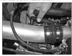
19. Vehicles equipped with an idle air vent line, install the 90 deg. fitting into vent line then mark the intake tube where the fitting lines up with tube.
