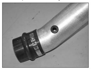
20. After marking the intake tube, remove from vehicle and drill a 7/8" hole into the intake tube then install the provided grommet as shown.
