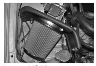
25. Install the K&N® air filter onto the mass air adapter and secure with the provided hose clamp as shown.
