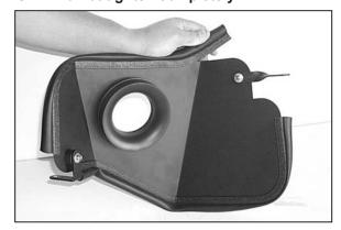
15. Install the twist bracket and the "L" bracket assembly onto the heat shield assembly with the provided hardware. Also install the trim seal onto the heat shield as shown.
