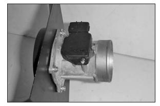
12. Assemble the mass air adapter, heat shield, gaskets and the mass air sensor using the hardware provided.
