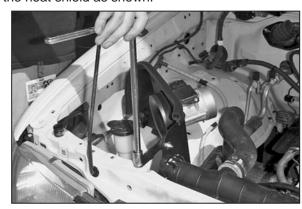
16. Install the heat shield assembly into the vehicle and secure it to the original air box mounting location as shown. Do not tighten completely.
