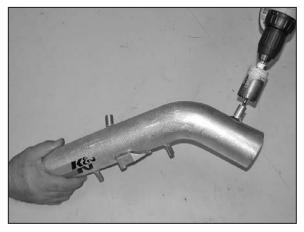
8. On vehicles equipped with the crank case resonator chamber, using a 1-3/8" hole saw, drill out the 5/8" vent port as shown.
