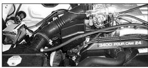
3. Disconnect the three hoses from the air box resonator and intake hose.
