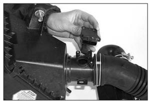
11. Loosen and remove the screws that secure the mass air sensor, then remove the mass air sensor.
