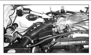
Loosen the hose clamps at the throttle body.
