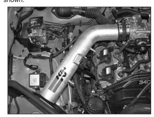
19. Install the K&N® intake tube onto the throttle body and align with the tube mounting bracket installed in step #16. Secure the tube with the provided hardware to the mounting bracket and tighten the hose clamp at the throttle body.
