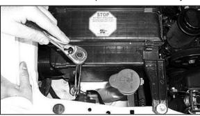
5. Loosen the three bolts that retain the air box assembly.
