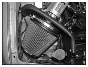
26. <u>Install the air filter</u> assembly onto the K&N<sup>®</sup> intake tube and secure with the provided hose clamp.
