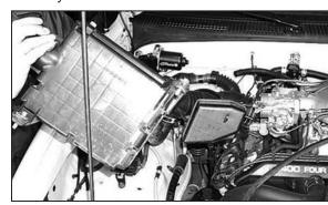
6. Remove the complete air intake system.
