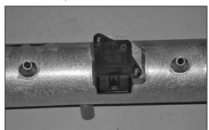
12. Install the mass air sensor into the K&N® intake tube and seucre with the provided hardware.
