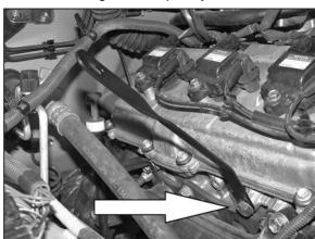
16. Install the tube-mounting bracket onto engine with the supplied hardware as shown.
