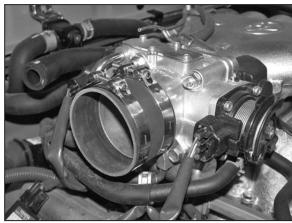
18. Install the silicone hose (08440) onto the throttle body with the provided hose clamps as shown.
