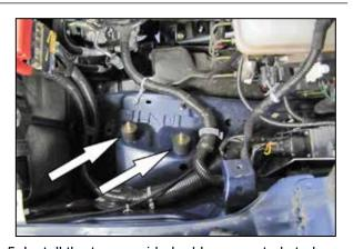
5. Install the two provided rubber mounted studs into the air filter housing mounting locations as shown.
