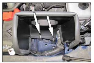
9. Set the heat shield onto the rubber mounted studs installed previously and secure with the provided nuts and washers.
