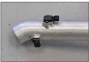
14. Install the sensors into the K&N® intake tube and secure with the provided hardware.
