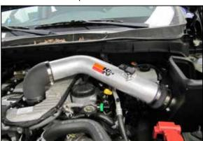
15. Install the K&N® intake tube into the coupler at the filter adapter and then into the hose at the turbo inlet, adjust the tube for best fit and then secure with the provided hose clamps.
