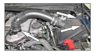
3. Loosen the hose clamp that secure the intake tube to the turbo inlet and then release the two clam shell clips that secure the upper air filter housing. Remove the upper air filter housing and intake tube from the vehicle.
