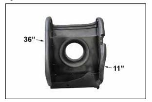
8. Install the edge trim onto the heat shield as shown.
