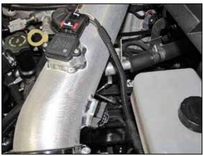
15. Reconnect the mass air sensor and inlet air temperature sensor electrical connections.
