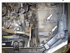
9. Remove the two airbox mounting studs shown from the inner fender.
