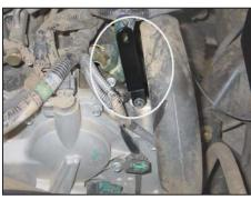
17. Install the tube mounting bracket (07191) onto the engine and secure with the factory bolt removed in the previous step.
