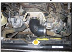
18. Install the provided silicone hose (084095) onto the throttle body and secure with the provided hose clamp.
