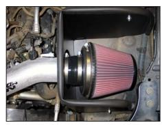
28. Install the filter assembly onto the K&N® intake tube and secure with the provided hose clamp.
