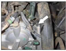
16. Remove the engine ground strap mounting bolt shown.
