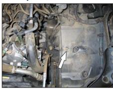
14. Remove the ground strap mounting bolt shown. **NOTE: this bolt will be reused in the next step.**
