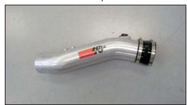
21. Install the provided silicone hose (08051) onto the  $K\&N^{\otimes}$  intake tube as shown and secure with the provided hose clamp.
