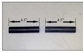
22. Cut the provided crankcase vent hose into two 4.5" sections as shown.
