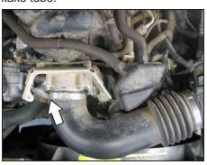
6. Loosen the hose clamp which secures the intake tube to the throttle body.
