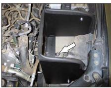
15. Install the heat shield assembly into position and secure with the provided hardware and the bolt removed in the previous step.
