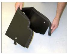
13. Install the provided edge trim onto the heat shield as shown.
