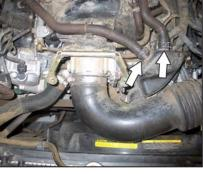
5. Release the two spring clamps which secure the crankcase vent hoses to the intake tube and then disconnect the crankcase vent hoses from the intake tube.
