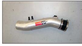
24. Install the two  $1\!\!\!/_4$  NPT crankcase vent fittings into the K&N® intake tube as shown.
