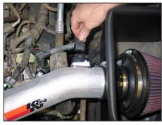
29. Reconnect the mass air sensor electrical connection.
