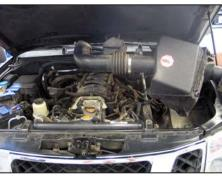
8. Remove the complete intake assembly from the vehicle as shown.
