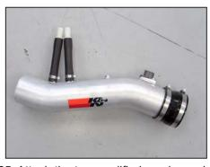
25. Attach the two modified crankcase hoses onto the  $\ensuremath{^{1}\!\!\!/}$  NPT fittings.
