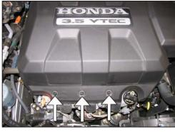
2. Turn the three engine cover retaining screws 1/4 turn counter clockwise to unlock the cover from the engine.
