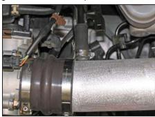
21. Install the provided silicone vent hose onto the K&N intake tube and then install the crank case vent tube into the silicone hose as shown. Secure the vent hose to the K&N® intake tube with the provided hose clamp as shown.
