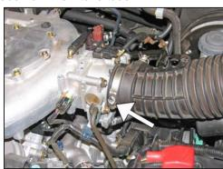
6. Loosen the hose clamp, which secures the intake tube to the throttle body.
