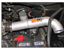
20. Install the K&N® intake tube into the silicone hose at the throttle body so that the mounting bracket rests on the heat shield mounting bracket and the mounting tab on the strut tower. Secure the mounting bracket to the heat shield bracket and mounting tab with the provided hardware and tighten the hose clamp at the throttle body.
