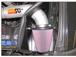
22. Install the K&N® air filter onto the intake tube as shown, and secure with the provided hose clamp.
