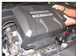
3. Lift the engine cover up to dislodge it from the mounting grommets and then remove it from the engine as shown.
