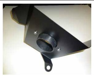
3. Install the radius filter adapter into the heat shield and secure with the provided hardware.
