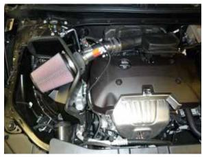
14. Reconnect the vehicle's negative battery cable. Double check to make sure everything is tight and properly positioned before starting the vehicle.
