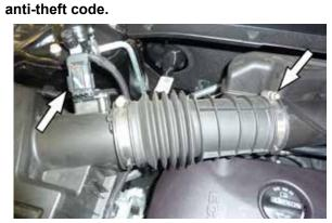
2.Disconnect the mass air sensor electrical connection and loosen the hose clamp that secures the intake hose to the plenum. Pull straight up and remove the complete air filter housing assembly from the vehicle. NOTE: K&N Engineering, Inc., recommends that customers do not discard factory air intake
