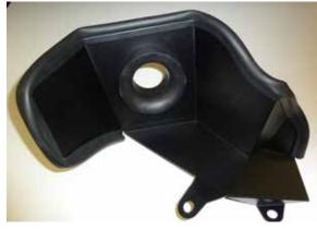
4.Install the edge trim onto the heat shield as shown. **NOTE: Some trimming of the edge trim may necessary.**
