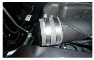
8. Install the provided straight coupler onto the intake plenum and secure with the provided hose clamp.
