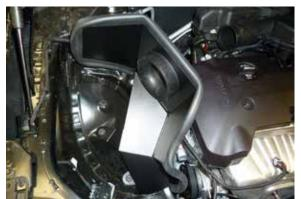
6. Install the heat shield assembly onto the mounting studs as shown.
