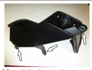
5. Remove the three factory mounting grommets from the factory air filter housing and install them into the K&N heat shield as shown.
