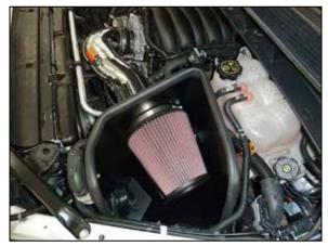
26. Install the K&N<sup>®</sup> air filter onto the adapter and secure with the provided hose clamp.
