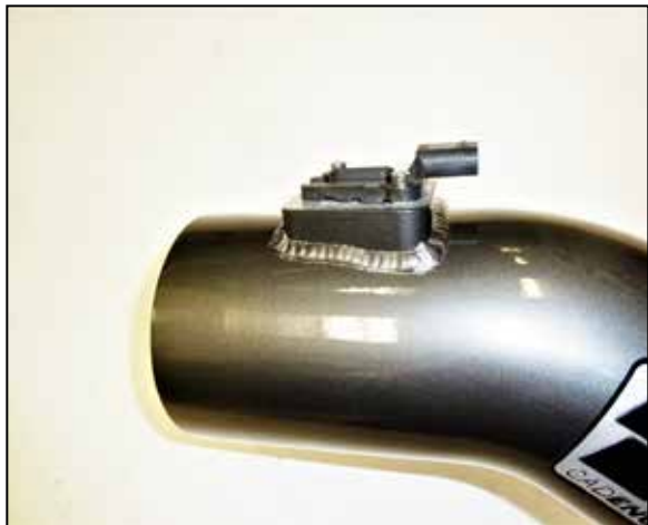
10. Remove the mass air sensor from the factory air filter housing and install it using the provided hardware.
