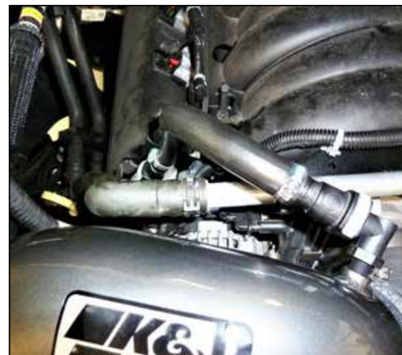
19. Connect the CCV hose assembly to the valve cover and intake tube fittings.
