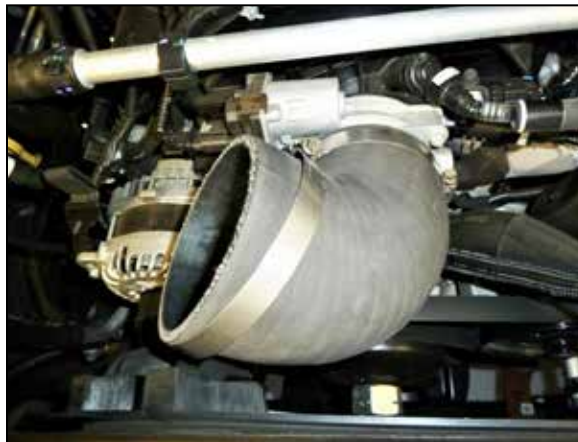
15. Install the angled coupler onto the throttle body but do not tighten the hose clamp at this time.
