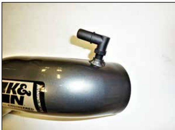
11. Install the provided 90deg quick connect fitting into the K&N intake tube as shown.
