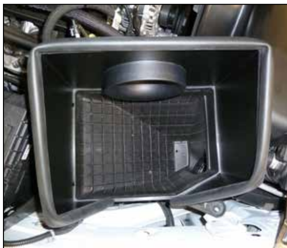
14. Install the heat shield assembly onto the factory lower air filter housing and secure with the seven screws provided.
