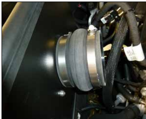
16. Install the hump coupler onto the filter adapter and secure with the provided hose clamp.
