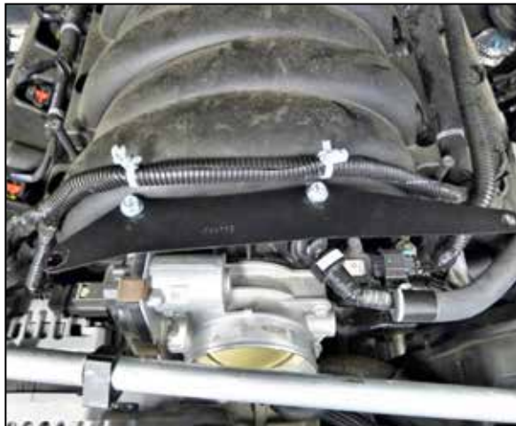
8. Install the provided mounting bracket onto the intake manifold using the provided hardware.
