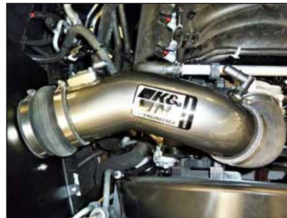
17. Install the intake tube into the couplers, adjust the coupler and tube for best fit and then secure with the provided hose clamps.
