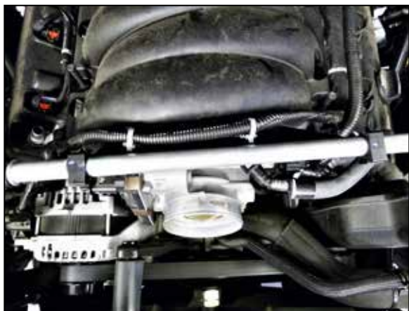
9. Secure the wiring harness and coolant pipe to the mounting bracket as shown.
