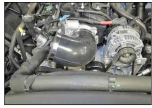
16. Install the provided coupler hose (084086) onto the throttle body but do not completely tighten at this time.
