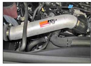
17. Install the K&N® intake tube into the coupling hoses and then adjust the tube for best fit. Secure the hoses and tube with the provided hose clamps.
