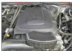
2. Lift up and remove the engine cover from the engine.
