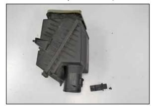
12. Remove the screws securing the mass air sensor into the air filter housing and then remove the sensor.
