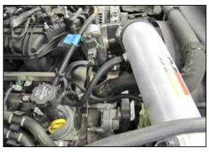
18. Install the provided crank case vent hose onto the fitting installed into the K&N® intake tube and then onto the valve cover port. Secure the hose to the valve cover port with the provided hose clamp.
