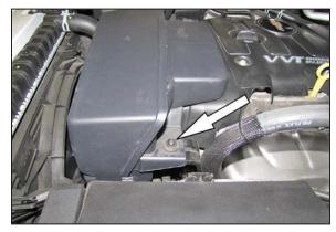
3. Remove the bolt that secures the intake plenum to the engine.
