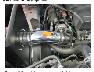
19. Install the Intake tube assembly into the coupling hose at the filter adapter and then connect it to the throttle body, adjust the tube, hoses and heat shield for best fit and then secure with the provided hose clamps and hardware.
