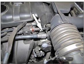
4. Disconnect the crank case vent hose from the intake plenum.
