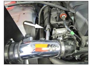
20. Connect the crank case vent hose to the fitting installed into the K&N $^{\! \rm 8}$  intake tube.
