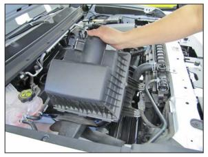
8. Remove the air filter housing assembly from the vehicle.
