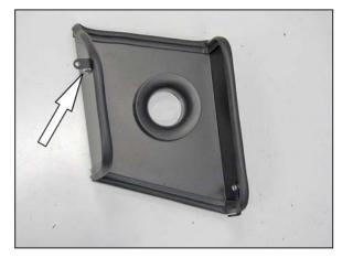
13. Install the heat shield mounting bracket (07805) onto the heat shield using the provided hardware and spacer.
