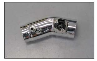
16. Install the mass air sensor into the K&N® adapter and then install the assembly into the K&N® intake tube and secure with the provided hardware.
