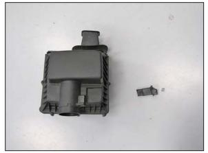
15. Remove the two screws securing the mass air sensor and then remove the mass air sensor from the factory air filter housing.
