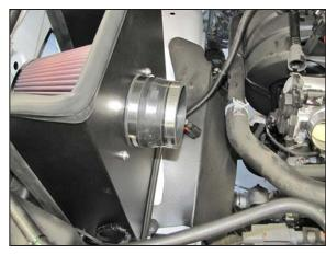
17. Install the provided coupling hose (08051) onto the filter adapter and secure with the provided hose clamp.
