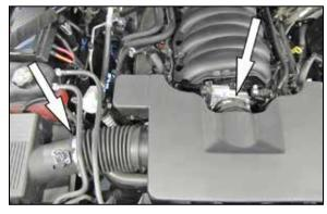
4. Loosen the two hose clamps securing the intake plenum to the factory air box and to the throttle body.
