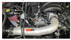
18. Install the K&N® intake tube into the hose at the filter adapter and then into the hose at the throttle body, adjust the tube for best fit and then secure with the provided hose clamps.
