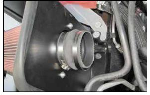
14. Install the coupling hose (08699) to the filter adapter and secure with the provided hose clamp.
