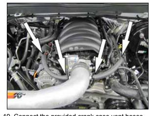
19. Connect the provided crank case vent hoses to the ports on the valve covers and then connect the open ends to the fittings installed into the K&N® intake tube.
