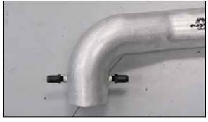
17. Install the two provided crank case vent fittings into the  $K\&N^{\otimes}$  intake tube as shown.
