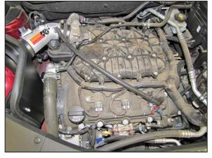
25. Install the crank case vent assembly onto the valve cover port and then onto the fitting installed into the K&N<sup>®</sup> intake tube as shown.
