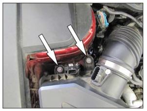
6. Loosen and remove the two bolts securing the air filter housing to the inner fender.
