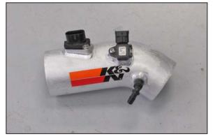
18. Install the 90° vent fitting into the K&N<sup>®</sup> intake tube as shown.
