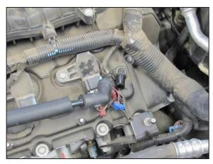
22. Remove the crank case vent tube from the valve cover port.
