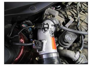
27. Reconnect the mass air sensor and humidity sensor electrical connections. NOTE: Some vehicles may not be equipped with a humidity sensor.
