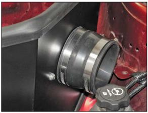
10. Install the remaining "L" bracket (070066) onto the heat shield as shown using the provided hardware.
