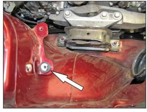
14. Install the remaining rubber mounted stud onto the air box mounting bracket as shown.
