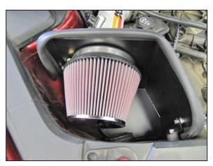
26. Install the K&N<sup>®</sup> air filter onto the filter adapter and secure with the provided hose clamp.
