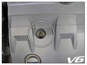
2. Remove the bolt securing the engine cover, remove the oil filler cap and then lift off the engine cover and remove it from the engine. NOTE: reinstall the oil filler cap.
