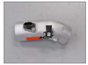
17. Install the mass air sensor and humidity sensor into the K&N<sup>®</sup> intake tube using the provided hardware.
