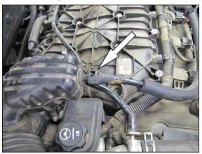
4. Disconnect the crank case vent tube from the intake plenum.
