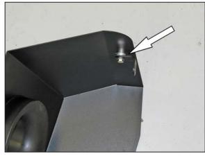
9. Install one of the provided "L" brackets (070066) onto the heat shield as shown using the provided hardware and spacer.
