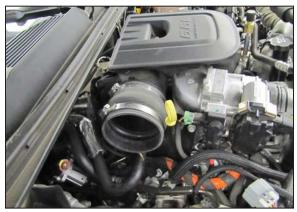
14. Install the provided hump hose (08633) onto the turbo inlet pipe and secure with the provided hose clamp.
