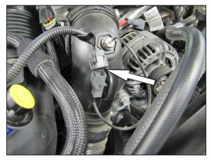
2. Disconnect the wiring harness junction connector located on the intercooler charge tube.
