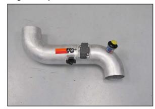
19. On vehicles that are equipped with a filter minder, install the provided grommet and the factory filter minder into the K&N<sup>®</sup> intake tube as shown. On vehicles not equipped with a filter minder, Install the provided plug.
