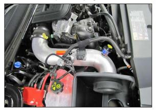
20. Install the K&N<sup>®</sup> intake tube into the hump hose at the turbo inlet and then into the hose at the filter adapter. Align the tube for best fit and then secure with the provided hardware.
