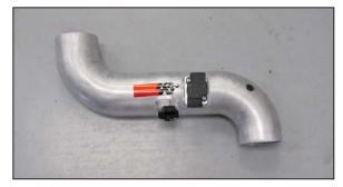
18. Install the MAF sensors into the K&N<sup>®</sup> intake tube and secure with the provided hardware.
