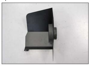
9. Install the filter adapter into the K&N<sup>®</sup> heat shield as shown using the provided hardware.
