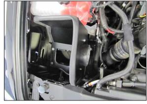
13. Install the K&N<sup>®</sup> heat shield onto the air box mounting plate and secure with the factory bolts from step #8.
