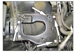
8. Remove the three bolts and the grommet shown from the air box mounting plate. **NOTE: These bolts will be reused in a later step.**
