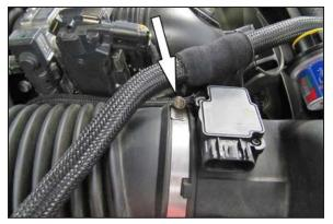
4. Loosen the hose clamp that secures the intake tube to the factory air box.
