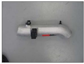
16. Install the sensors into the K&N® intake tube and secure with the provided hardware.
