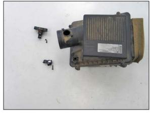
15. Remove the screws securing the mass air sensor and pressure sensor into the factory air box lid and then remove the sensors.
