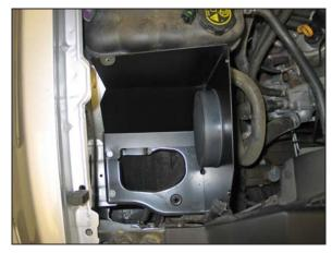
12. Install the heat shield onto the air box mounting plate and secure with the provided hardware to the factory mounting locations.
