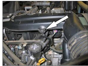
4. Disconnect the crank case vent hose from the intake tube plenum.
