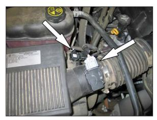
2. Disconnect the mass air sensor and pressure sensor electrical connections shown.
