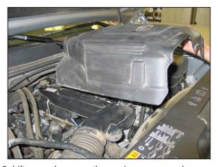
3. Lift up and remove the engine cover as shown.
