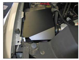
22. Install the air box lid and secure with the provided hardware.
