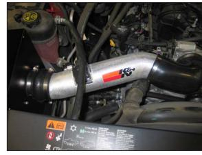
18. Install the K&N® intake tube assembly onto the filter adapter and then the throttle body. Adjust the tube and hose for proper fit and then tighten the hose clamps.
