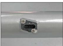
16. Install the mass air sensor into the K&N<sup>®</sup> intake tube and secure with the provided hardware.
