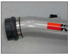
18. Install the provided silicone hose (5-576) onto the  $K\&N^{\circledR}$  intake tube as shown.
