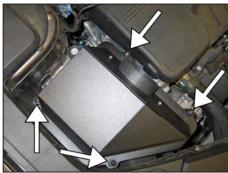
13. Secure the K&N® upper airbox with the four screws removed in the previous step.
