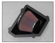
10. Install the K&N<sup>®</sup> air filter onto the filter adapter and secure with the provided hose clamp.
