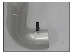
17. Install the provided vent fitting into the  $K\&N^{\circledR}$  intake tube as shown.
