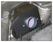
11. Set the K&N<sup>®</sup> upper airbox assembly onto the factory lower airbox as shown.
