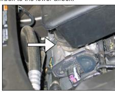
5. Loosen the hose clamp securing the intake plenum to the throttle body.
