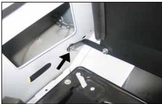
19. Secure the mounting bracket to the inner fender with the hardware provided. NOTE: Be sure to place one fender washer on each side of the inner fender.
