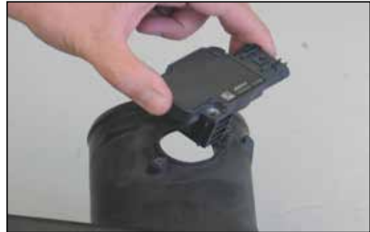
9. Remove the two screws securing the mass air sensor to the air box and then remove the mass air sensor from the air box as shown.
