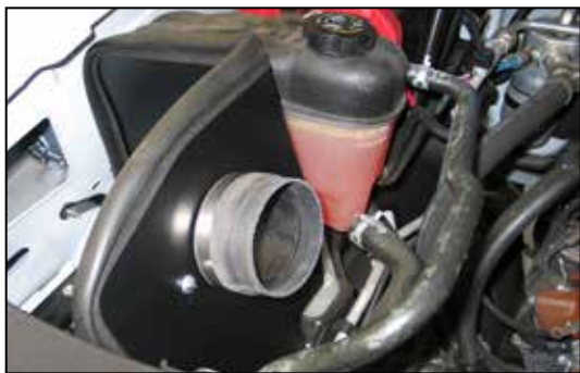
21. Install silicone hose (#084057) onto the filter adapter and secure with the provided hose clamp.
