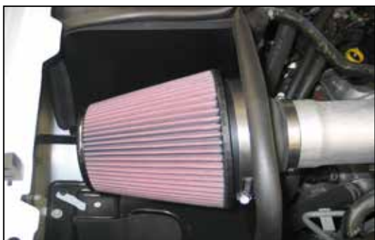
26. Install the K&N® air filter onto the filter adaptor and secure with the provided hose clamp. NOTE: Drycharger® air filter wrap; part # RF-1042DK is available to purchase separately.
