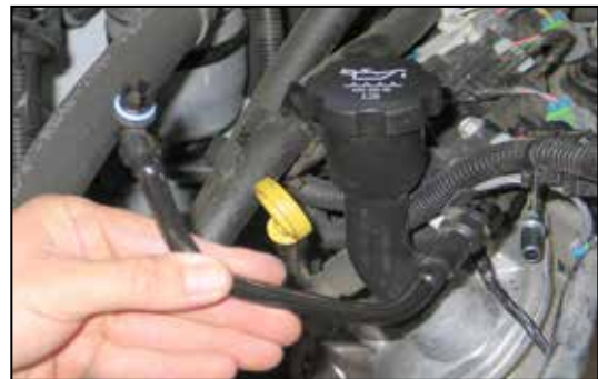
7. Rotate the crank case vent line on the valve cover port, and then release the locking tab and remove the crank case vent line from the valve cover.
