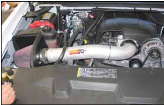
29. Reconnect the vehicle's negative battery cable. Double check to make sure everything is tight and properly positioned before starting the vehicle.
