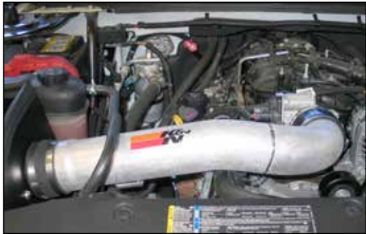
24. Install the K&N® intake tube into the silicone hose at the filter adapter and then into the silicone hose at the throttle body, then secure with the provided hose clamps.
