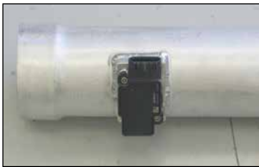
10. Install the mass air sensor into the K&N® intake tube and secure with the provided hardware.
