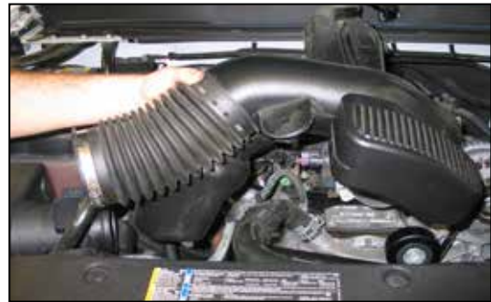
6. Loosen the hose clamp, which secure the stock intake tube, then remove the intake tube from the vehicle.
