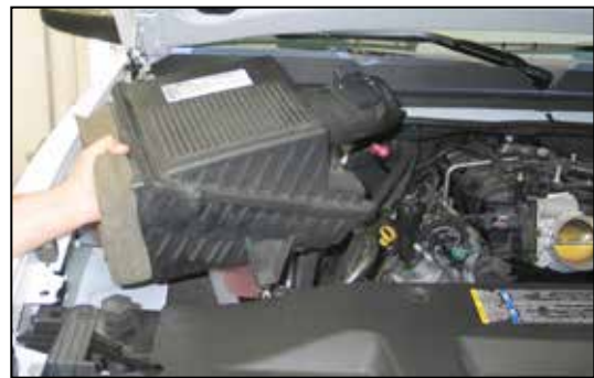
8. Pull firmly upward to release the air cleaner assembly from the mounting tray grommets. Then remove the assembly as shown. NOTE: K&N Engineering, Inc., recommends that customers do not discard factory air intake.
