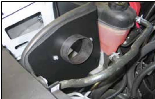
20. Install the filter adapter onto the heat shield and secure with the provided hardware.
