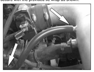
23. Install the provided crank case vent hose onto the valve cover and then onto the K&N<sup>®</sup> intake tube as shown.
