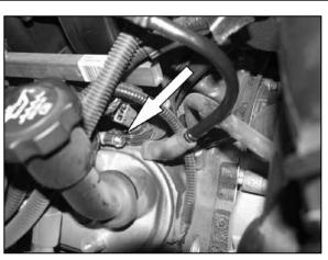
5. Disconnect crankcase vent hose from the valve cover as shown.
