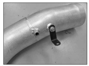
20. Install the "L" bracket (070812) onto the  $K\&N^{\otimes}$  intake tube with the provided hardware as shown.
