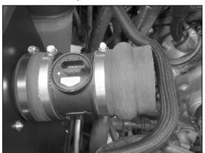
19. Install the silicone hump hose (08176) onto the  $K\&N^{\odot}$  intake tube and secure with the provided hose clamp as shown.
