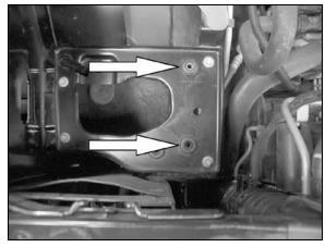
12. Remove the two air box mounting grommets shown.
