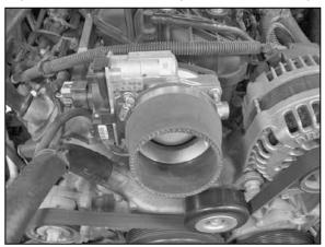
17. Install the silicone (08050) hose onto the throttle body and secure with the provided hose clamp.
