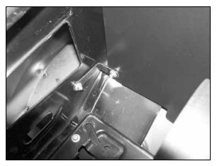
15. Secure the heat shield mounting bracket to the inner fender with the fender washers and hardware as shown.
