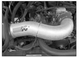
21. Install the K&N® intake tube into the silicone hose at the throttle body and mass air sensor and secure it with the provided hose clamps.
