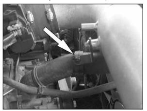
22. Install the upper radiator hose mount onto the "L" bracket installed onto the K&N® intake tube and secure with the provided tie wrap as shown.
