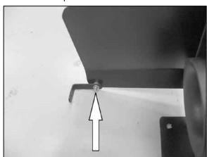
10. Install the "L" bracket (010031) onto the heat shield with the provided hardware as shown.
