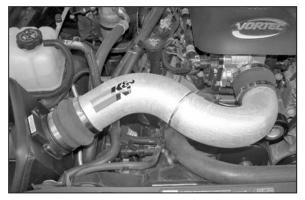
13. Install the K&N<sup>®</sup> intake tube onto the mass air sensor, then secure the other end onto the throttle body as shown.
