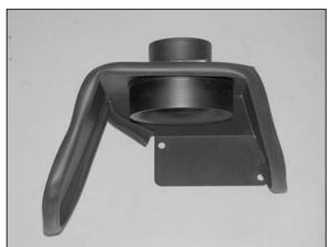
9. Assemble the mass air adapter, heat shield, gaskets and the mass air sensor as shown above.
