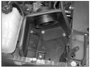
10. Install the heat shield assembly onto the rubber mounted studs using the hardware provided.
