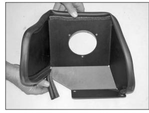
8. Apply the trim seal to the heat shield assembly as shown.
