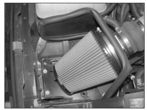
15. Install the K&N<sup>®</sup> air filter onto the heat shield assembly as shown.
