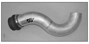
12. Install the silicone hump hose (08176 ) and hose clamps onto the K&N $^{\mbox{\tiny ($0$}}$  intake tube as shown.
