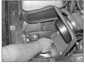
14. Adjust the heat shield and intake tube for best fit, then tighten the two nuts as shown.
