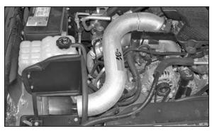
15. Install the K&N<sup>®</sup> intake tube into the silicone hose at the intake inlet, then align the tube to the mounting bracket installed in step #7 and secure with the provided hardware.
