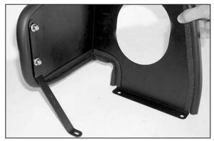
9. Install bracket onto heat shield as shown. Do not tighten completely.
