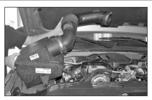
4. Lift up on the air box assembly to release from the mounting grommets, and then remove the air box and intake tube assembly from the vehicle. NOTE: K&N Engineering, Inc., recommends that customers do not discard factory air intake.
