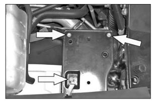
10. Remove the three bolts from the stock airbox mounting tray.
