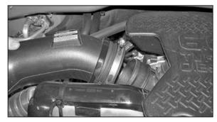
3. Loosen the hose clamp, which secures the intake tube to the intake manifold, and then disconnect the intake tube from the intake manifold.
