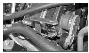
7. Using the factory bolt removed in step #6, install the tube mounting bracket to the engine processor as shown.
