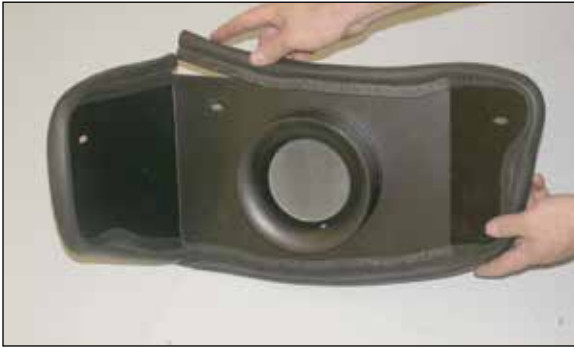
11. Install the edge trim onto the heat shield. Trim if needed.
