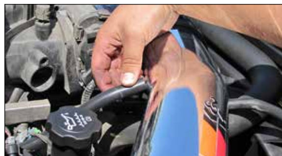
20a. On vehicles equipped with a crank case vent, install the provided crank case vent hose to the valve cover port and then align the hose to the K&N® intake tube in the straightest possible location. Mark this location on the intake tube and then remove the tube.
