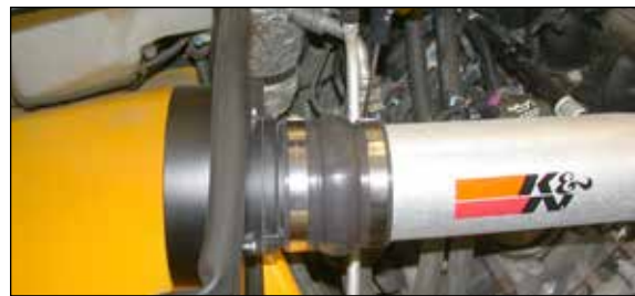
20. Install the K&N® intake tube assembly onto the throttle body and into the silicone hose attached to the mass air sensor, then tighten the hose clamp to secure at the mass air sensor.
