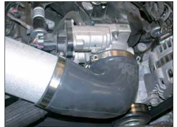
21. Tighten the hose clamp, which secures the silicone hose to the throttle body.
