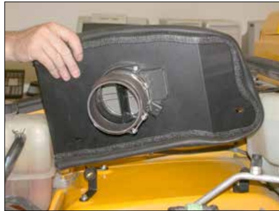
17. Install the heat shield assembly into vehicle as shown.
