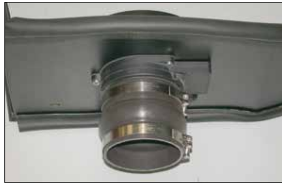
16. Install the silicone hose (084053) onto the K&N® intakes tube as shown using the supplied hose clamps.
