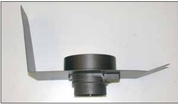
10. Install the mass air sensor and filter adapter onto the heat shield using the gaskets and hardware provided.
