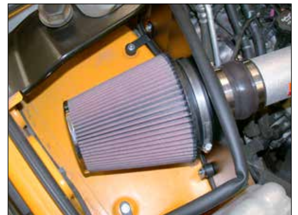
22. Install the air filter onto the mass air sensor and then tighten hose clamp.
