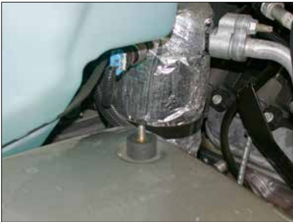
14. Install the rubber mounted stud (07027) onto the vehicle as shown.
