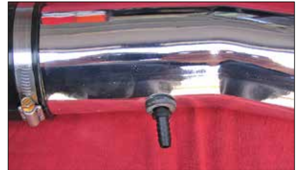
20c. Install the provided grommet and hose mender into the K&N® intake tube as shown.
