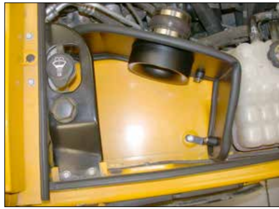
18. Secure the brackets to the heat shield with the provided hardware. Do not tighten completely.
