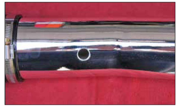
20b. Drill a 5/8" id hole at the location marked on the intake tube during the previous step. Be sure to remove any burrs or shavings after drilling the hole into the intake tube.
