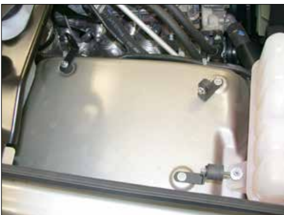
15. Install the 3 brackets onto the vehicle with the provided hardware as shown. Don't tighten completely at this time.
