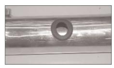
16c. Use a 1-1/4 hole saw to drill a hole where the intake tube was marked in the previous step. Then install the provided grommet as shown.
