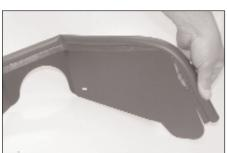
10. Install the trim seal onto the heat shield and trim to fit as shown.
