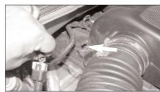
4. Unclip the air temperature sensor harness
