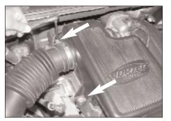
6. Loosen the two bolts on the resonator as shown.
