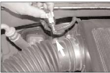
3. Remove the air temperature sensor from the stock intake tube as shown.
