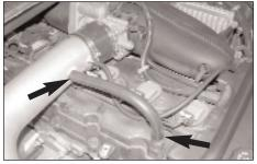
19. Install the provided silicone hose onto the vent on the K&N® intake tube and connect the other end to the crank case vent on the cam cover as shown.
