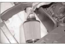
20. Install the K&N® air filter onto the K&N® intake tube and secure using the provided hose clamp as shown.
