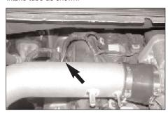
17. Install the air temperature sensor into the grommet on the K&N® intake tube as shown.
