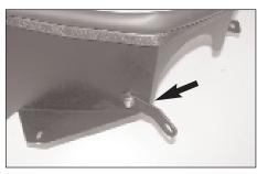
11. Install the provided bracket onto the heat shield using the provided hardware but do not tighten completely at this time.
