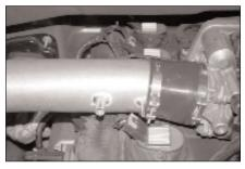
15. Slide the K&N® intake tube into the silicone hose at the throttle body as shown.
