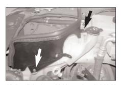
12. Install the heat shield onto the windshield washer reservoir and secure to the stock air cleaner cover mounting holes using the provided hardware but do not tighten completely at this time.
