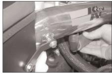
16b. On vehicles with air injection, install the 90 degree fitting into the vent line then mark the intake tube were the fitting lines up with tube, then remove intake tube from vehicle.
