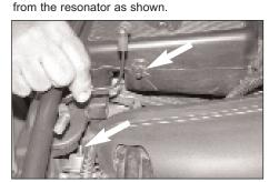
5. Remove the vacuum hose from the fuel pressure regulator and from the resonator as shown.
