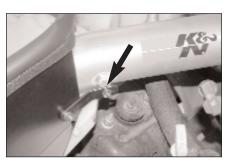
16. Secure the bracket on the heat shield to the threaded boss on the K&N® intake tube. Check everything for best fit and clearance then tighten all hose clamps and hardware.
