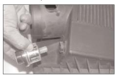
19. Remove the stock restriction gauge from the stock air cleaner as shown.
