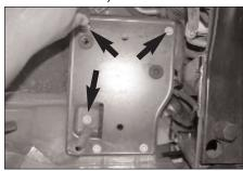
9. Remove the three air cleaner support tray bolts as shown.
