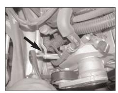
10. Remove the air conditioning hard line bolt
