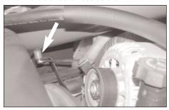
18. Line up the twist bracket from step 11 with the threaded boss on the K&N® intake tube and secure with the provided hardware as shown.
