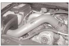
17. Slide the K&N® intake tube through the hole in the heat shield, then, slide the other end of the tube into the silicone hose as shown.
