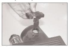
Remove the mass air sensor from the stock air cleaner assembly as shown.
