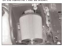
23. Install the K&N® Air Filter onto the K&N® intake tube and secure with the provided hose clamp as shown.
