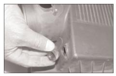
20. Remove the grommet from the stock air cleaner as shown.
