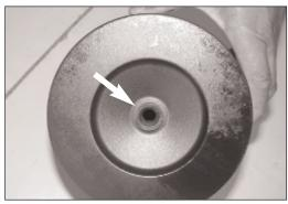
21. Install the grommet from step 20 into the hole on the end of the K&N® Air Filter as shown.
