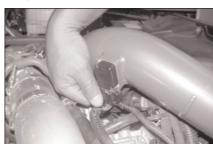
24. Reconnect the mass air sensor electrical connection as shown.
