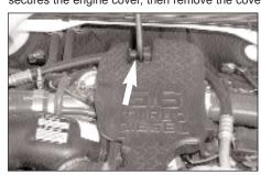
4. On 2002 models remove the torx bolt from the intake resonator as shown.
