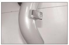
16. Install the mass air sensor into the K&N® intake tube and secure with the provided screws as shown.
