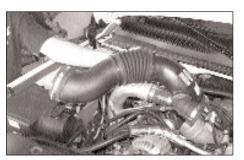
6. Loosen the hose clamp at the intake manifold and at the air cleaner then remove the stock intake tube as shown.
