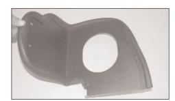
12. Install the provided trim seal onto the K&N® heat shield and trim to fit as shown.
