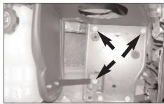
14. Install the heat shield into the vehicle and secure with the stock bolts from step 9 as shown but do not tighten completely at this time.
