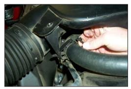
4. Unclip the radiator hose from the stock intake tube as shown.
