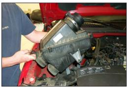
6. Pull firmly upwards to remove the air cleaner assembly as shown.
