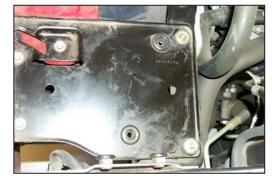
9. Install the rubber mounted studs as shown and tighten firmly by hand.
