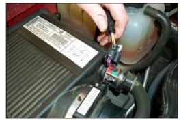
3. Disconnect the mass air sensor electrical connection as shown.
